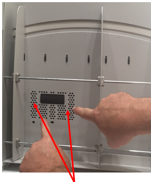
Drilled Vented Holes
